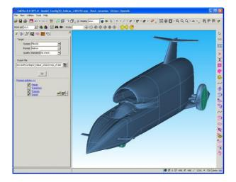
In addition to facilitating a direct interface to the complex NX design geometry, the CADfix integration meant that specialist CADfix geometry processing functions, such as the suppression of unwanted small features and the correction of poor surface parameterisations, could be applied to ensure that the optimum geometry was available for FLITE meshing and analysis.
